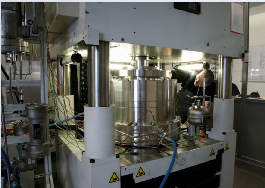
Seals up to approx. 800 mm can be tested, and the process conditions simulated, on our own test facilities. Shown here a 1.5 metric tons seal of the EagleBurgmann HSH series.
